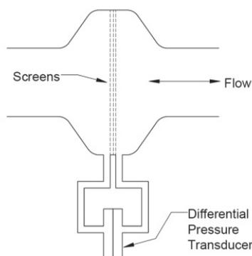
Figure 1. Differential Pressure Pneumatich
